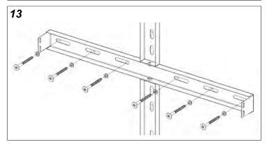
For each additional battery (up to three) in the stack, screw in the vertical spacer to the last horizontal retainer installed. Repeat steps 1 through 3 for each horizontal retainer, as shown in Figure 14 (for studs) or 15 (for concrete).
