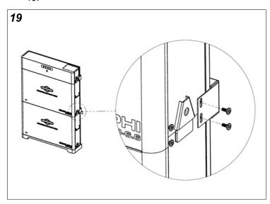
4. If applicable, repeat steps 1-3 to install the second battery module on top of the first and the third battery on top of the second. See Figure 20.
