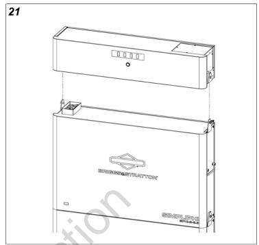
This completes installation of the SimpliPHI 6.6 BESS. Continue to Conduit Installation (outdoors) or Electrical Wiring Installation (indoors).
