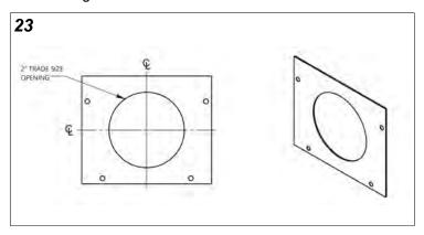
Install the conduit chase nipple or appropriate outdoor rated fitting onto the side plate. See Figure 24.
