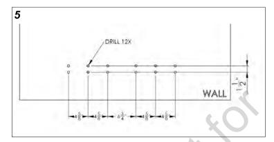
As required by the fastener manufacturer's recommendations, use the appropriate drill for the material to pre-drill holes on the wall in the specified positions.
