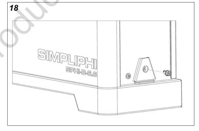
3. Reinstall the rear shoulder screws into the battery through the slot on the wall retainer, as shown in Figure 19.
