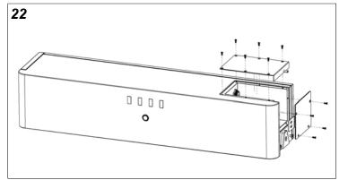
2. Choose the appropriately sized conduit, up to 2" trade size maximum, for your cables per local AHJ and NEC installation requirements.
